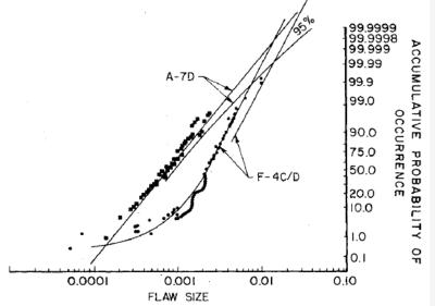
Fig. 11 Cumulative probability of occurrence of A-7D and F-4C/D equivalent initial quality.
